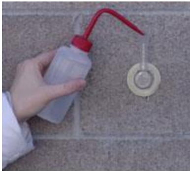
Figure 1. Karsten tube absorption test.
