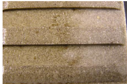
Fig. 2. The area dusted with SG-APS was rinsed after two hours and the petroleum engine oil was found to have disappeared.
