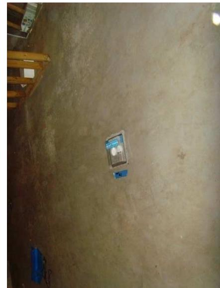
6. Leave test in place for 72 hours. After test is completed, remove the cover carefully with a stiff spatula. Close the capsule carefully and re-tape the capsule with the original blue tape (see step 2). Fill in the blanks on the right side of the capsule. Also record the PH level. Mail the capsule only to ReUse Concrete Sealing.
