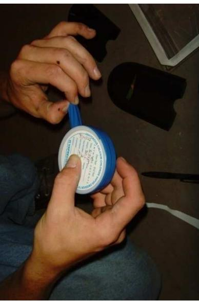
2. Hold container firmly (as in the picture) and remove blue tape carefully. Do not spill or open capsule.
