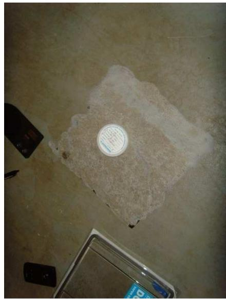
4. Fill in the blanks on the left side of the container (time and date). Place container on floor in the middle of the clean area and open carefully.
